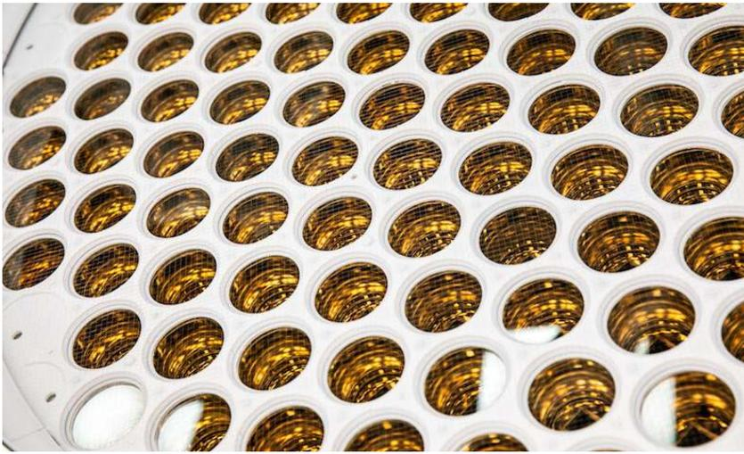
Photomultiplier tube arrays are prepared for the WIMP-hunting LUX-ZEPLIN experiment during assembly at the Sanford Underground Research Facility in Lead, South Dakota. Credit: Matt Kapust/SURF
