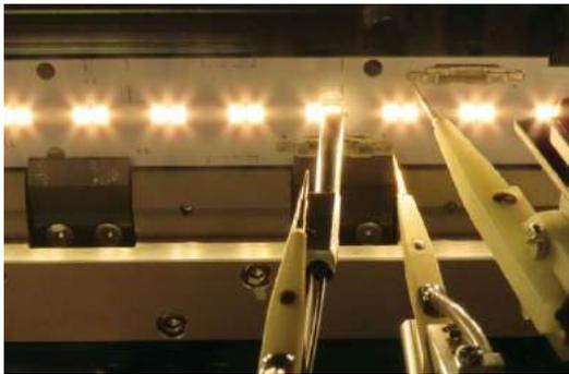
This is a FEASA sensor which can be installed on one or more heads, and can test the featuring settings of a Led: colour, intensity and saturation. FEASA is a renowned manufacturer of sensors which are globally acknowledged as the standard for Led characterization.
