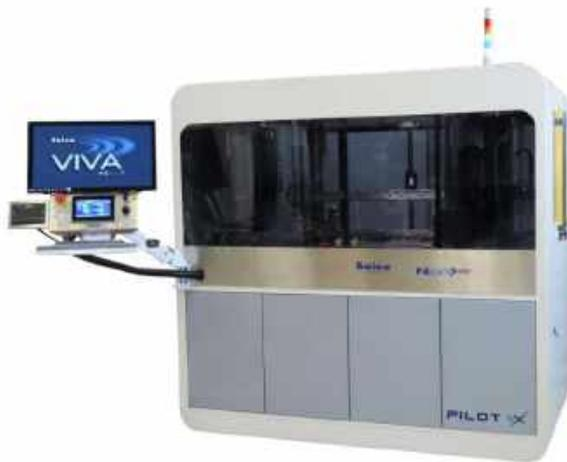
The Pilot VX has a multitude of new hardware and software features included, all aimed at addressing the fundamental concerns of electronic board manufacturers looking to optimize their investment. Time is cost, and the new state-of-the-art mechanical performance and motion control enables a reduction of up to 50% in test time. The Pilot VX has 12 multi-function test heads providing the
