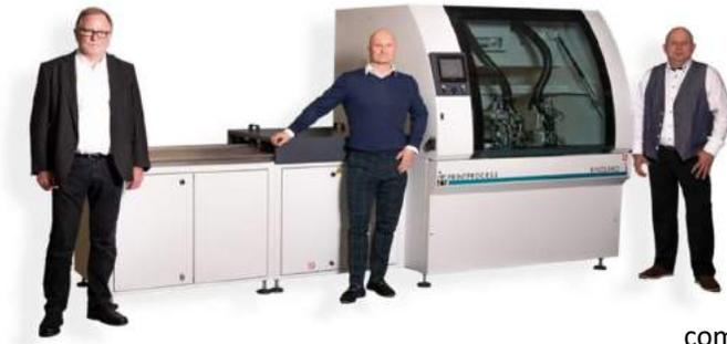
RIVOLINO layup system and the OPAL optical alignment system. Overall, there are many combinations of the production of multilayer boards with high-layer count and design complexity as well as exposure systems. The units are modular build so one could start with a manual system and upgrade to a fully automatic. The focus is the registration on each machine and their approach to find best fit for costumers manufacturing process.
